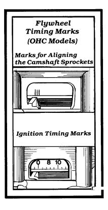
necessary, then paint it white. Paint two vertical lines on the top front of the crank pulley. OK, Picasso, put away the paint and brush. Remove the socket and ratchet from the pulley bolt.
