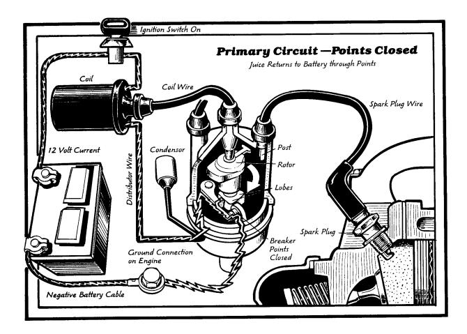
circuit winding (a wrapping of wires) inside the coil, then through a wire to the closed switch in the distributor, then to the distributor body, then back to the negative (-) battery terminal through the body of the car. As the juice passes through the primary winding of the coil, a concentrated electromagnetic field is created. High school science, remember?
