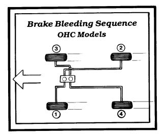
Condition: Brake pedal feels spongy or mushy and it takes a few pumps on the pedal before any braking action occurs; OR some part of the hydraulic system has been opened for inspection or repair.
