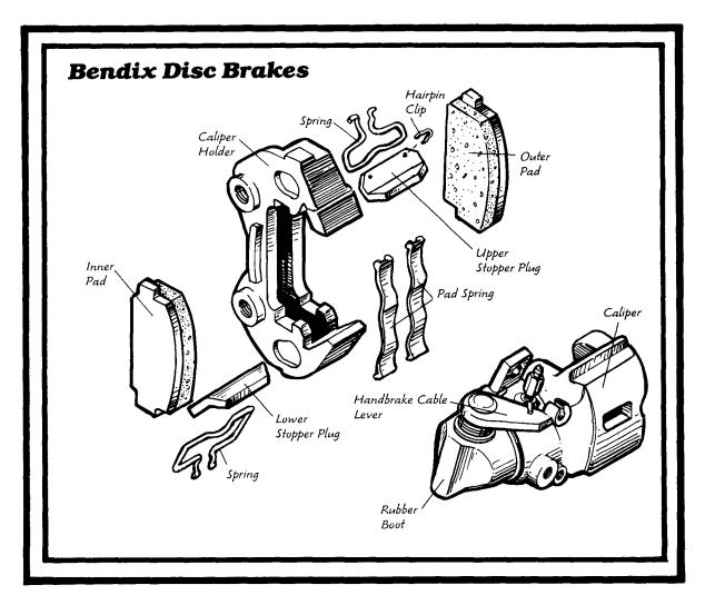
of the new pads to those on the old pads. The new pads should be free to move in the caliper holder without binding. They shouldn't be so loose they rattle either. A nice, lightly snug fit is just right. If the pads are too tight, return them for some that fit. Pads from the Subaru dealer usually fit the first time around.
