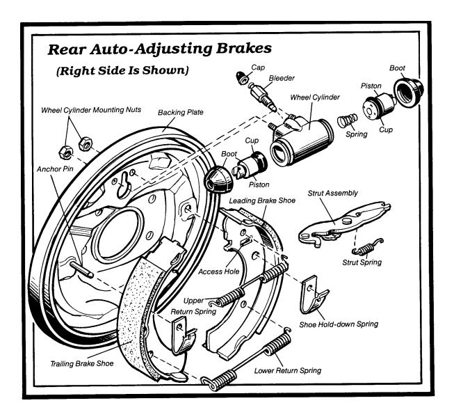
in the slots on the ends of the wheel cylinder and adjuster or anchor where the ends of the brake shoes fit. Wipe off excess grease with a rag.
