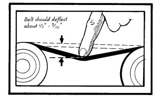
it between the two pulleys that are farthest apart.) Subaru says to use 22 lbs. of pressure. You'll have to guess how hard you're pushing (or maybe use a fisherman's spring scale and pull on the belt with 22 lbs. of force) while you measure the distance the belt deflects. To make things simple, use two fingers and push a bit harder than you push a doorbell. A new belt should deflect about'/z" and a used belt about 9/16".
