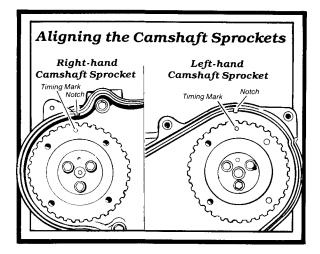
Install the long, left-hand belt first. If you are using the old belt, find your arrow and install the belt so the arrow is pointing toward the left side of the car.
