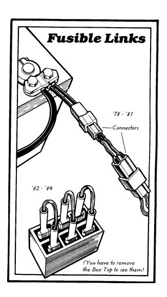
covered wires with a plastic connector on each end. To check the wires in the link, feel along the cloth on each wire to see if the wire is still intact. Sometimes the cloth will be burned and black at the point where the wire melted. The fusible link is a unit, so if one of the wires is burned or broken you have to replace them both. Be sure the new link has the proper rating for your year and model.
