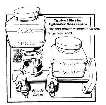
CAUTION!: Brake fluid is like a magnet for moisture in the air. An open can of brake fluid can become contaminated within a  $f_{ew}$  minutes on a humid day. So keep the can of brake fluid tightly sealed and the reservoir caps on except when adding fluid.
