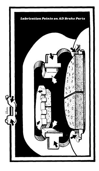
Late AD type: Follow the instructions for ventilated discs, above, to lubricate the lock pin, boot, and sleeve. Tighten the lock pin to 25 ft. lbs.
