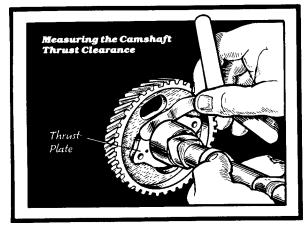
Inspect the teeth on the cam gear for chips, cracks, and wear. The machinist can help you with this. If the gear is worn out or damaged but the cam shaft is still good, you can have the machinist install a new cam gear.
