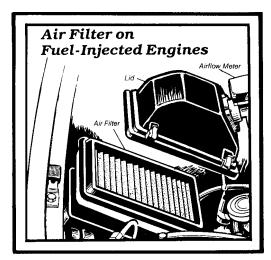
Carburetor models: The air cleaner is that large, blue or black, flat thing sitting on top of the engine. The parts of the air cleaner **are the top (or lid)**, a pleated paper **air filter element**, the larger bottom part **called the air filter housing**, **and a snout** that sticks out the right (passenger's) side of the housing. In 1980 the shape of the air cleaner changed from round to peanut shaped. First, take the lid off the housing.
