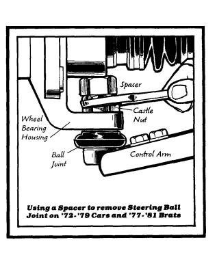
'75-'79 cars and '77-'81 Brats: Unscrew the three 17mm nuts that attach the bottom of the ball joint to the control arm. You'll have to hold the bolt heads with another 17mm wrench. Remove the three bolts, then push down on the control arm. If you're here to remove the ball joint, pull it out now.
