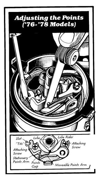
ratchet on the crank pulley bolt and rotate the engine *clockwise* until the lobe rider is exactly on the corner of one of the lobes so the points are opened up as far as they'll go.
