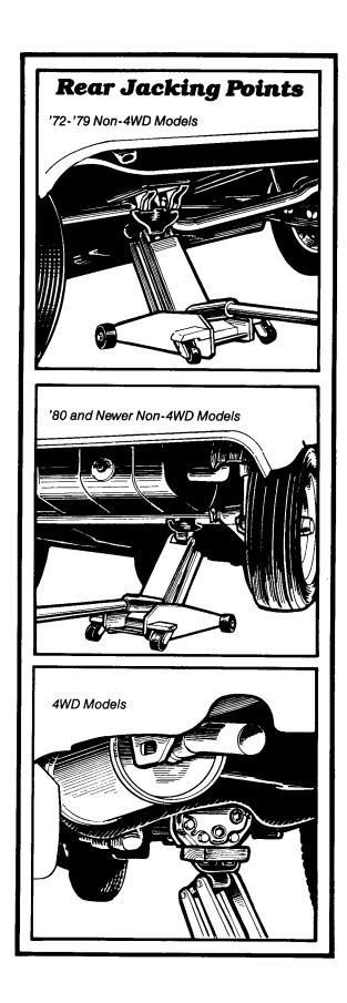
way, leave it in position for added safety. (If the jack handle is removable, remove it. If it isn't removable, be aware the handle's there, and try not to trip over it.) Check the bottoms of the jackstands to be sure they're squarely on the floor, not tilted.
