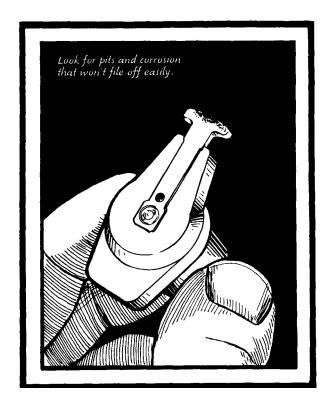
a new one (Step 10). If the cap is kaput and you're going to replace it, replace the rotor also.
