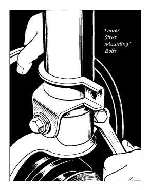
Step 2. Remove Lower Strut Mounting Bolts.
