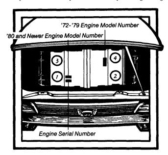
Engine Serial Number: Look on the top front of the engine, just to the right of center. You'll see a flat place with numbers stamped on it. That's the engine serial number.
