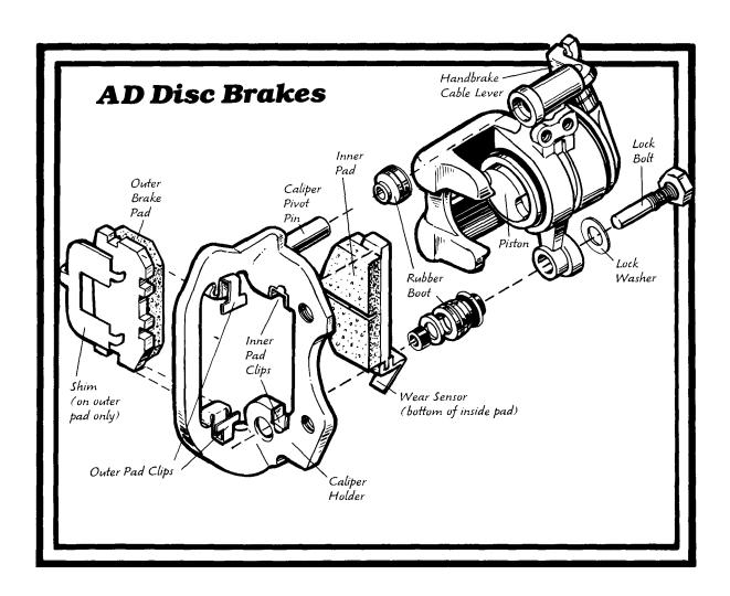
Step 4B. Screw Piston Into Caliper (no brake tool).
