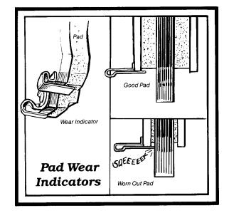
changing the brake pads and removing the caliper for repair or replacement is a breeze with either the Bendix or AD system. Rebuilding the calipers, especially AD calipers, is very tedious and difficult and should be left to the professionals.
