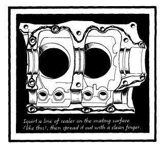
EVERYONE: Squeeze a bead of silicone gasket sealer on one of the case halves (as shown in the illustration), then use a clean finger to spread it into a thin layer that covers the entire mating surface. Don't get any sealer on the crankshaft.
