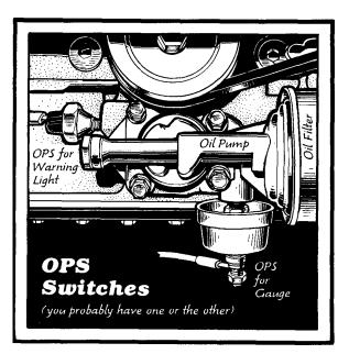
**B.** Check oil pressure switch (OPS): If you only have an oil pressure warning light on the dash (no gauge), the OPS will be screwed into the crankcase just to the right (passenger's) side of the oil pump. On models with an oil pressure gauge on the dash, the OPS is screwed into the bottom front of the oil pump near the oil filter.
