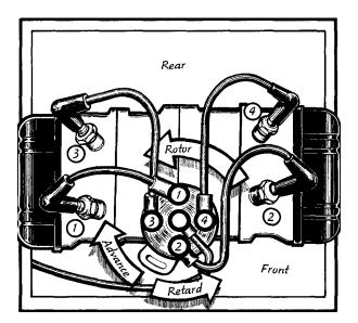
B2. Check spark plug wire connections, spark plugs, and engine compression: Are the spark plug wires securely connected to the distributor cap and spark plugs? Check 'em: push down on both ends of each wire. Remove the spark plugs and check their condition. Do a compression test while the spark plugs are out and evaluate the results. Directions for these checks are in Chapter 7, Procedure 11.
