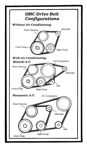
Some late models have a vertical 14mm bolt and lockwasher in a bracket just behind the upper idler pulley. If you have this bolt, turn the bolt *clockwise* to tighten the belt or *counterclockwise* to loosen it. If you're replacing the belt, loosen the bolt far enough that you can slip the belt off the pulleys, then install the new belt. Tighten the bolt until the tension is correct. Check the tension again after running the engine for about 15 minutes. Why aren't all belts this easy to adjust?
