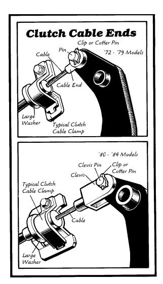
and stash the bolt and clamp where they won't get lost. Note how the large washers and rubber grommet on the end of the cable housing fit into a groove on the pedal bracket.
