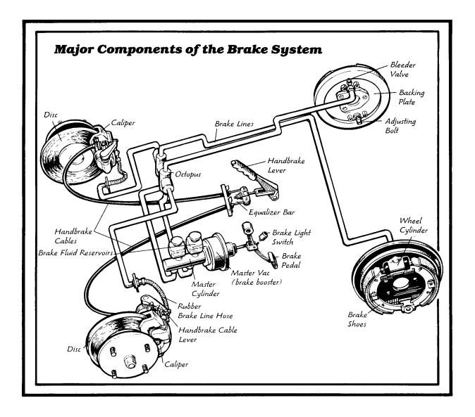
Each brake fluid reservoir cap has a switch that lights the brake warning light on the dash if the fluid level is low. Here's how your outside brake lights work: A switch for the brake lights is mounted to a bracket near the top of the brake pedal. When the pedal is pushed away from the switch the rear brake lights light up.
