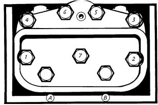
EVERYONE: Follow the cylinder head nut-loosening sequence to remove the other seven nuts and flat washers from each head. Put the nuts, bolts and washers, in a baggie labeled "Head Nuts."
