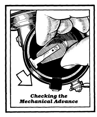
If the rotor doesn't snap back to its original position or if you can't turn the rotor, either the springs in the depths of the distributor are shot or there's junk down there. Do Step 7 to see if the circlip is loose and jamming the works. If it isn't, it's the springs and we can't fix them. They're set very carefully to comply with emission control standards. Have Subaru or an auto electric shop check and replace the springs if need be.
