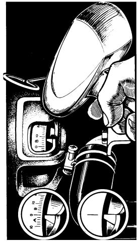
Engine set at TDC for adjusting valves for ', 1 and ti2 cylinders TDC for ,3 and --4 cylinders
