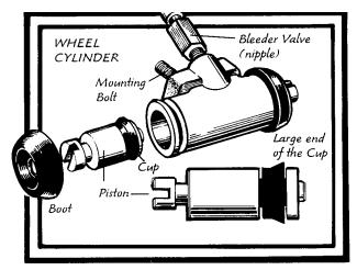
Put the rubber boots from each end of the wheel cylinder. As you remove the boot, out will come a piston with a rubber cup attached to the inside end. Note how the rubber cup is oriented on the end of the piston. The large flange on the cup faces toward the center of the wheel cylinder. On 1985 and newer models, a small spring will be in the cylinder, between the two pistons. Pull the spring out.
