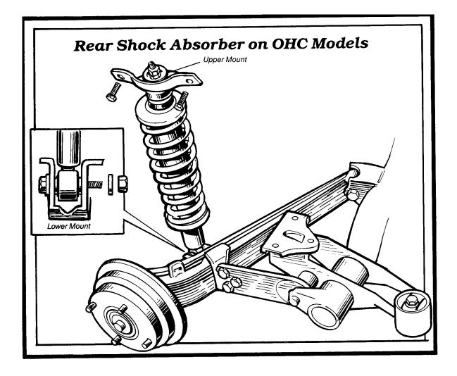
Step 3. Remove Lower Shock Mounting Nut or Bolt.
