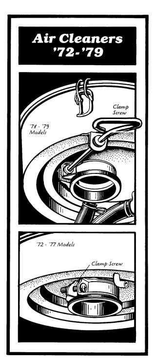
Attached to the bottom of the snoutlike air horn part of the air cleaner is a large, black or silver, **flexible hot air inlet hose.** To remove the hose, squeeze the two ears on the clamp and slide it down the hose. Grasp the hose as close to the air cleaner snout as possible and twist until it moves freely, then pull it off. It's fragile so squeeze gently. If the hose is torn or missing, make a note to get a new one.
