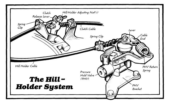
Condition 3: The hill-holder works fine on steep hills but not on moderate hills. Do Step 3, then Steps 1 and 2 if necessary.
