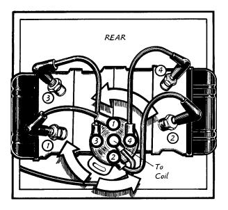
EVERYONE: Inspect the distributor cap and rotor (Chapter 7, Procedure 9, Steps 2 and 3). Replace them with new ones if they're getting funky. Use a Volt/Ohm meter to check the resistance of the spark plug wires (Chapter 10, Procedure 13). Replace them if the resistance values are higher than normal.
