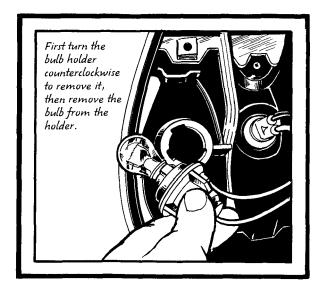
that matches the location of the nonworking bulb, twist the bulb holder counterclockwise (as viewed from inside the car) until it stops, then lift it out. See Step 2 of this procedure to change the bulb.
