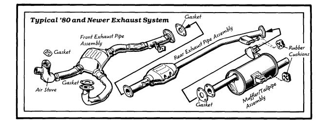
on top of your jack and slide it under the crotch. Raise the jack so it supports the weight of the pipe assembly (it's heavier than it appears).
