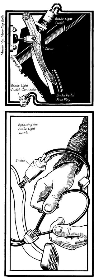
brake lights. If the brake lights are on, the brake light switch is bad. Replace it (Step 5). Still no lights? Either a wire is broken between the switch and brake light bulb, or the brake light system isn't grounded properly. See Chapter 10, Procedure 5.
