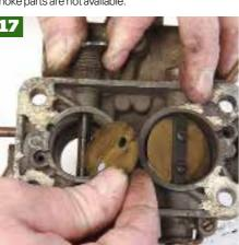
Undo the two screws that hold the butterfly in place and remove the butterfly. If they are tight gently tap with a hammer to loosen.
