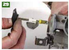
...then screw the choke unit to the main body, refit the choke pull-off diaphragm, and refit choke housing. If the old diaphragm was perished new items are available from Northampton Motorsport.
