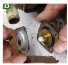
Now remove the accelerator diaphragm and enrichment device from the sides of the float bowl, and remove the mixer screw from the side of the main body. (Some DGAVs do not have the enrichment device).
