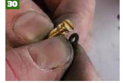
Next refit the mixture screw in the side of the main body, replacing the O-ring with a new item. To roughly get the right mixture wind the screw in all the way then unscrew by two turns.
