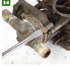
Remove the automatic choke housing (on the DGAV). If the unit works leave it alone as trying to repair them usually ends up with the centre bolt shearing off. If that happens the only way forward is to convert to manual choke as replacement auto choke parts are not available.
