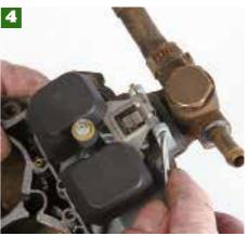
Then undo the six screws that hold the top on, and remove the top of the carb from the main body. Be careful as the screw heads are fairly soft metal.
