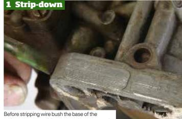
carburettor to reveal the part numbers stamped. These identify the carb and are needed to order the correct replacement parts. In this case it is a 32/36 DGAV '3D1'.
