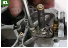
Refit the power valve diaphragm and float needle valve into the top of the carb then the filter with the new item from the service kit and replace 19mm filter nut. Once again new diaphragms are available.
