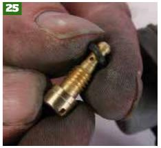
Before refitting the jets and emulsifying tubes replace the old O-rings with new ones from the service kit. Refit the jets in the same position you marked down earlier in step 9.
