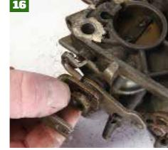
Turn the carb over to see the throttle butterflies. Remove the locking tab and 12 mm locking nut that holds the throttle shaft in position. Before removing the linkages and springs either write down or take a photograph of the order they come off in to help you remember how it all goes back together.
