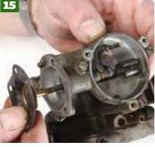
Then remove the three screws that hold the choke pull-off diaphragm in place and remove the diaphragm itself. Check it is in good condition, if not a replacement will be needed. Then remove the choke unit from the main body by undoing the three retaining screws at the side.
