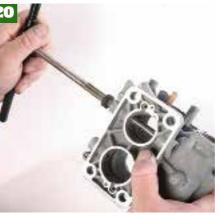
Before reassembling the carb Northampton Motorsport carry out a couple of trick mods. Firstly the base of the carb is machined totally flat to ensure a perfect seal with the spacer block. Also the body is reamed to accept Teflon bushes between the body and throttle shafts.
