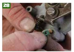
Refit the auto choke unit replacing the small green O-ring for the new one from the service kit...
