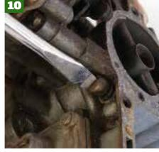
Remove the idle jet and progression jet from the sides of the float bowl.
