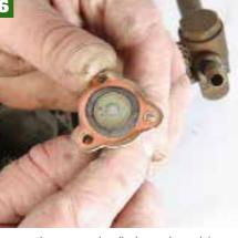
Remove the power valve diaphragm by undoing the three flathead screws that hold it in position, and take a closer inspection. This one's really had it.
