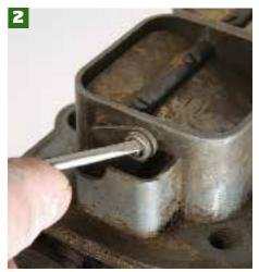
Now you can start stripping. Firstly remove the circlip for the choke butterflies with a small flathead screwdriver. Take care not to slip.
