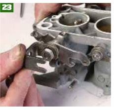
Refit the throttle butterflies and reassemble the throttle shaft linkages and springs in the reverse order to the way it was disassembled.
