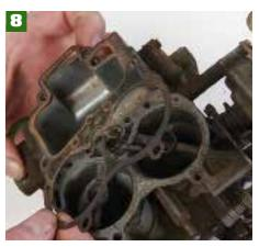
Now move on to stripping the main body of the carb. The first thing to go is the old gasket.
