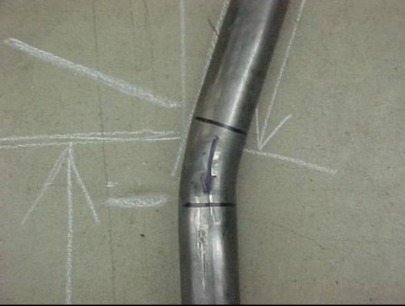
All that is left is to mark and cut it to the right height... You can use the same technique to do door bars front hoops on and on and on.... I know this is only single plain bends and very simple, but it should help you to get STARTED.
