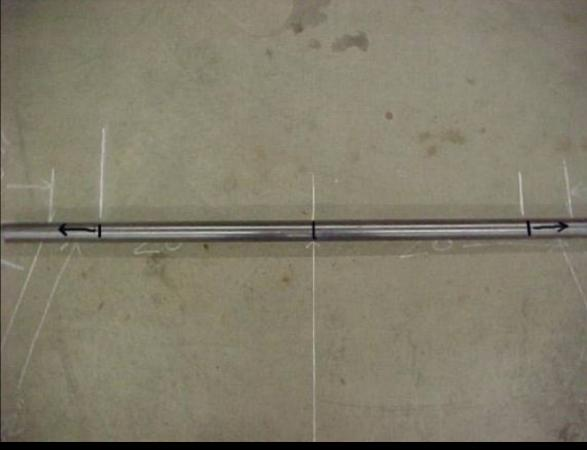
Chalk up your tube in the bender by lining up the marks and the direction arrow (seam to the inside).
