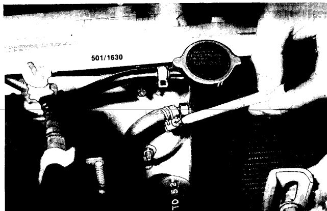
Ensure that the oil cooler hose clips are secure.
