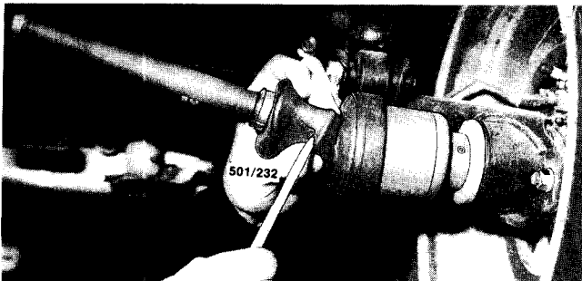
Check the axle shaft double offset joint rubber boot for signs of leakage, damage and deterioration.
