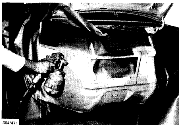
Applying spray putty to the repaired area.
