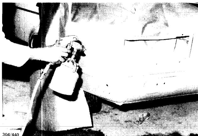
Applying the primer/surfacer to the repaired area.
