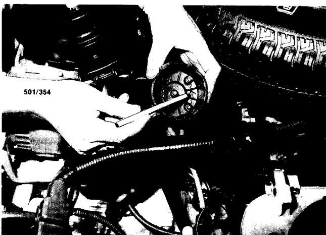
Check the distributor cap for cracks and tracking.
