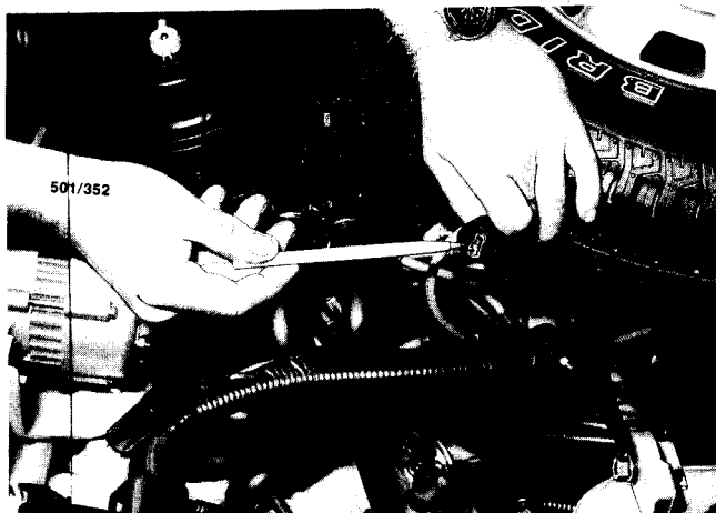
Check the high tension terminals for corrosion and burning.
