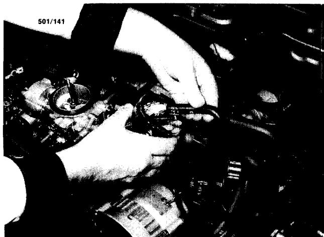
Check for fuel flow at the carburettor supply line.
