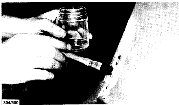
Applying the deoxidising agent/rust convertor to the rusted area.
