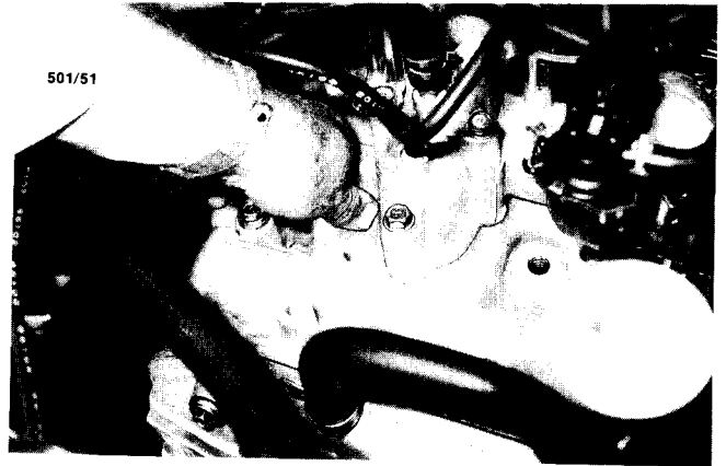
Check for compression by placing a thumb over the spark plug hole and have an assistant operate the starter.
