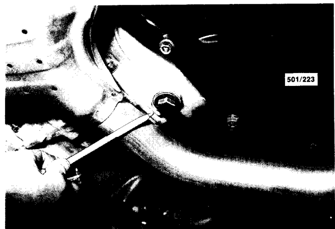
Location of the manual transaxle drain plug, 1986 model shown.
