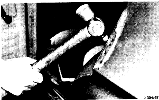
Using a ball pein hammer to tap down the rust affected area.
