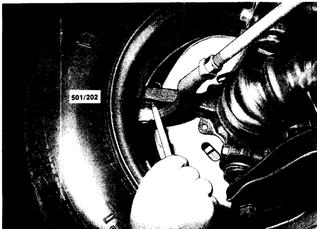
Check the tie rod end rubber boot for deterioration.
