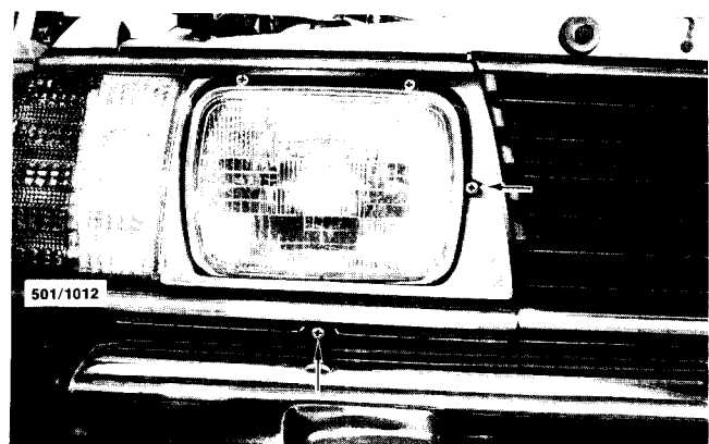
View showing the headlamp adjusting screws, 1981 model shown.
