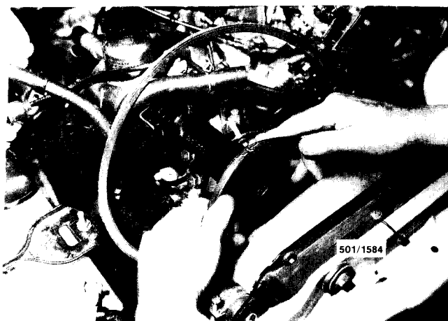
Checking the power steering pump drive belt for deterioration.
