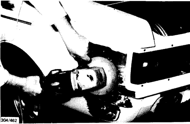
Removing the old paint finish from the damaged area using a disc sander.
