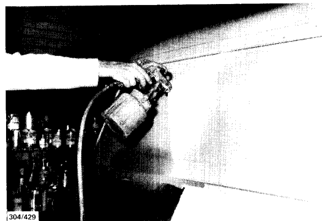
View of the spray gun held at the incorrect angle when spraying a vertical surface.
