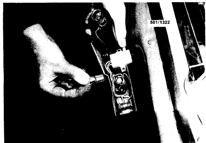
View showing the bulb holder and bulb removed from the rear combination lamp, 1983 Coupe shown.
