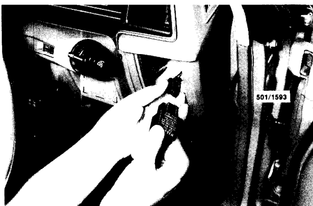
Remove the right hand trinket tray to gain access to the flasher unit on 1979–1984 models and all Utility models.
