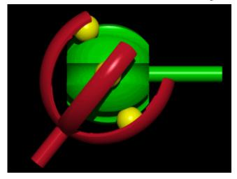
So, when you do a U-Turn, the Balls goes from one Side to Another very <u>very Fast</u>; if Acceleration is Forced (in Example while Accelerating the Engine) the Balls will go Faster and **harder** with the Extra **Pressure and shearing** against the walls, and that will **Worn** them and their Holding Basket very Fast, also their C.V. Joint's base.
